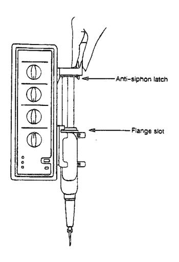
WARNING: ASSURE THE SYRINGE BARREL FLANGE IS PROPERLY INSERTED INTO THE HOLDER'S NOTCH OR UNCONTROLLED EMPTYING MAY OCCUR.
