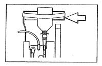
Vial or Syringe: Secure the container to the cassette door using the *optional* container support arm.
