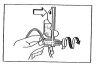
Turn the flow regulator until a drop of fluid is seen in the pumping chamber.
