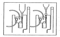
Attach the secondary container to the secondary inlet port (capped port shown on the left, prepierced port on the right).
