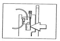
Confirm that the cassette air trap is full of fluid. If air is present, use the backpriming function to expel the air.
