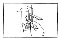
Holding the primed cassette by its fingergrip, slide it into the cassette door guides until it firmly seats in the door. Close the cassette door.
