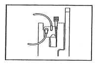
Primary only: Remove the container attached to the secondary inlet port, then cap the port (if appropriate).
